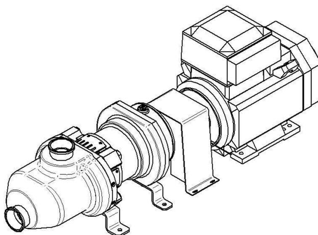
**Fig. 3 – Pump on baseplate**
