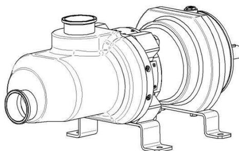
**Fig. 2 – Bare-shaft pump**
